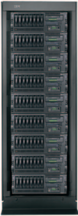
IBM 7014 Model T00 rack with nine pSeries 615 Model 6C3 drawers.
